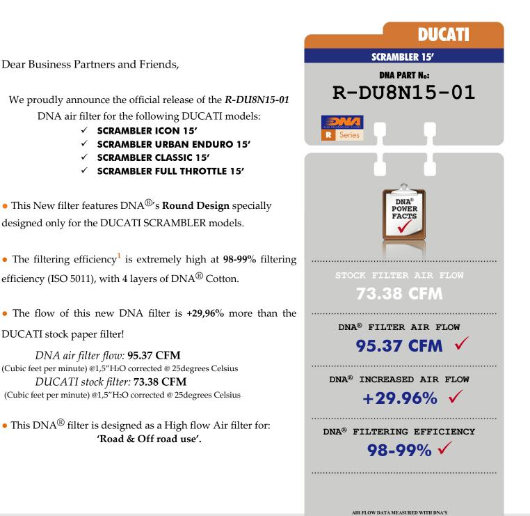
AIR FLOW DATA MEASURED WITH DNA'S ROTRONICS FLOWSCAN COMPUTERIZED FLOWBENCH
