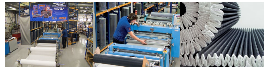
100% organic cotton filtering media, combined with epoxy coated marine grade aluminum wire mesh.
